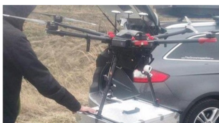
A multirotor drone carrying a frequency-spectrum measurement payload — a practical tool for measuring coverage where drive or walk tests cannot reach. (Source: Study 18)
